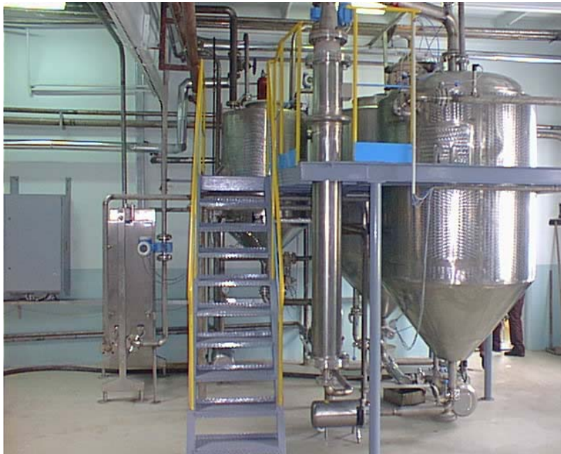
Compact design of a molasses treatment plant
