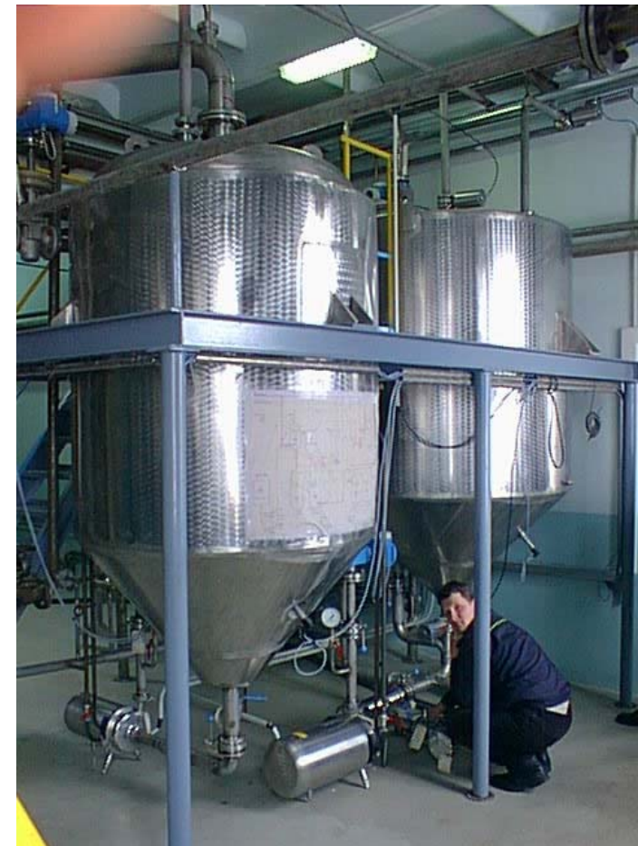
Compact design of a molasses treatment plant
